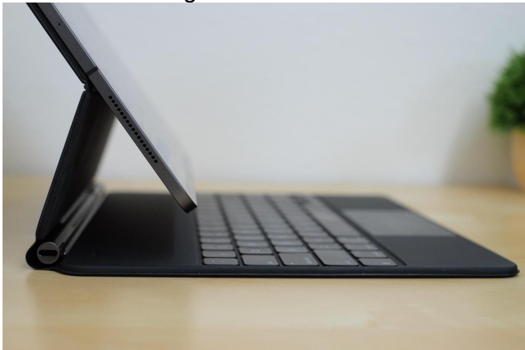
The Magic Keyboard's hinge has a USB-C port for charging the iPad Pro. Jason Cipriani/ZDNet
